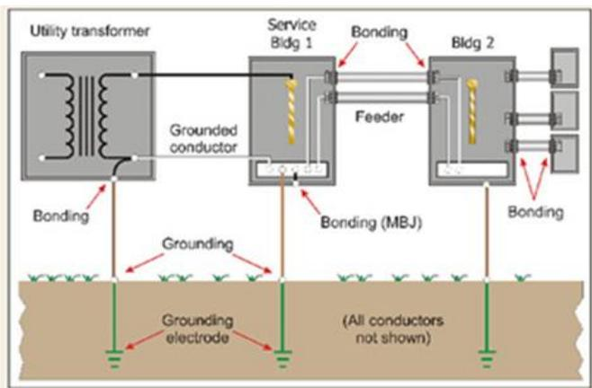
Fig.2 Grounding and bonding functions
