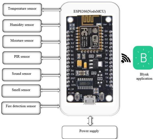
If the value exceeds the threshold, we get blynk email and blynk notification. Based on the notification, we can take precautionary measures, blynk mobile application used to see parametric values remotely.
