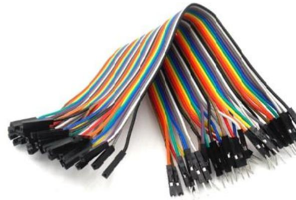
**Gambar 4 Kabel Jumper**
